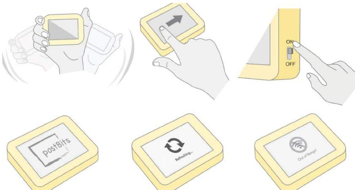
**Fig. 2** Interacting with *PostBits* by **a** shake **b** swipe and **c** switch ON/OFF. Shaking the *PostBit* will **d** reset a *PostBit*, Swiping will **e** refresh the display and **f** if the *PostBit* is out of range it displays the message
