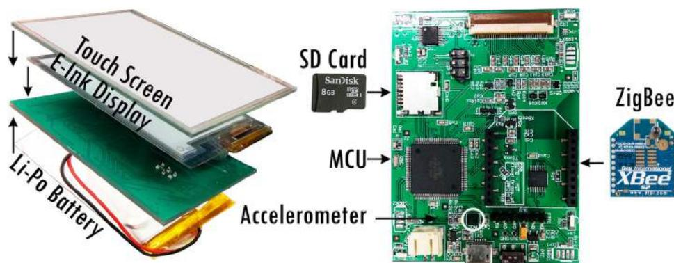
refreshed, the screen draws 10 mA. Once the image is set, E-Ink technology is able to hold it indefinitely without any energy consumption. Basic user interaction consumes very low energy consumption. When activated the touch screen shows a consumption peak of 780  $\mu$ A and accelerometer continuously drains 47 $\mu$ A. This set-up provides approximately 8 days of continuous operation with a 2000-mAh battery.
