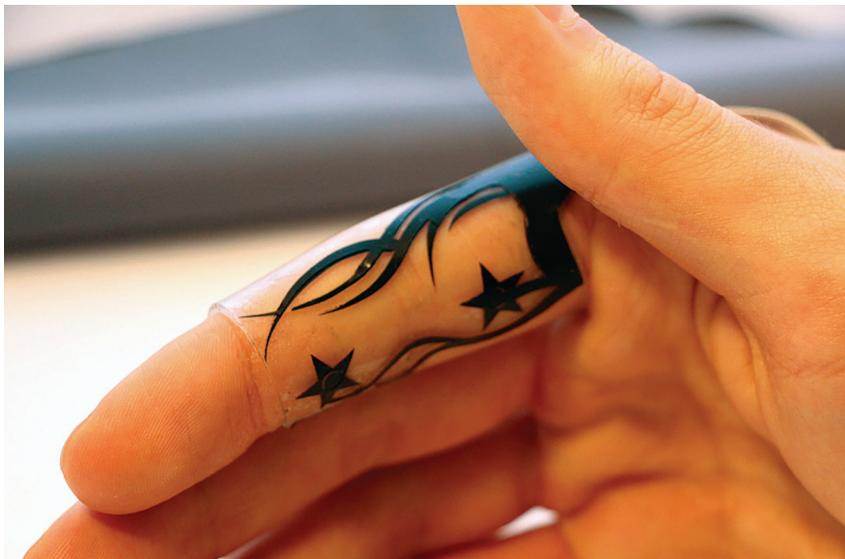
**Figure 3.** Aesthetic on-skin devices. The iSkin touch sensor is thin and stretchable. Using digital fabrication, it can be customized to fit the user's aesthetic preferences and individual proportions so it can be worn at various locations on the body.
