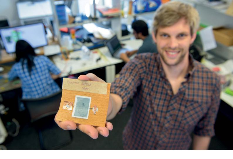
Prototypes: Doctoral student Simon Olberding holds up a thin, light-emitting display that the scientists printed onto wood using the PrintScreen technique. The display detects the user's touch input through the veneer. This method was also used to enhance a conventional Swatch wristwatch by printing the display onto the band with symbols that alert the user – for example when a new e-mail has been received.
