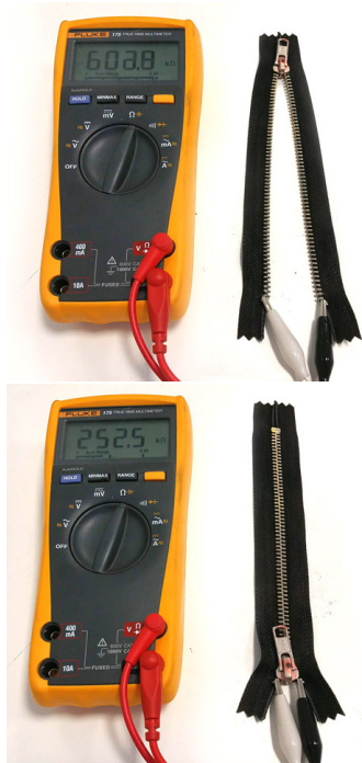
Figure 7: A polymerized zipper can sense its own state. When open, the resistance is high because the path travelled is long. When closed, the resistance is low, as electricity can flow through the zippers teeth.
