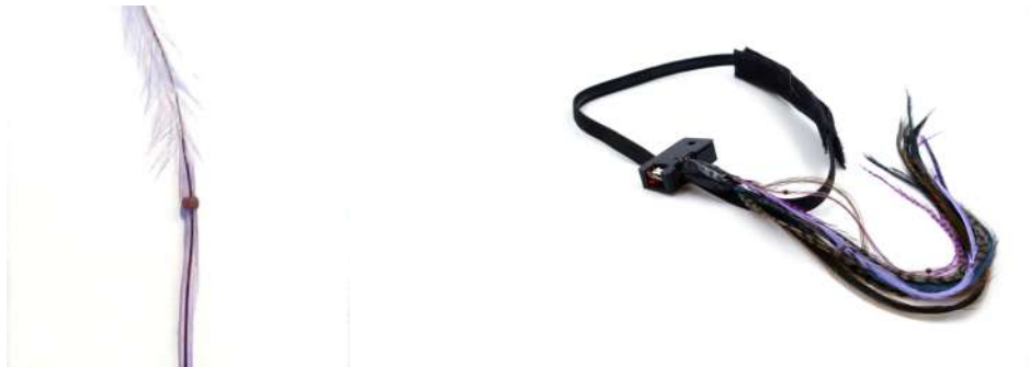
Figure 3.8: Left: One of the beads attached to the feathers in order to provide haptic feedback. Right: The final prototype with integrated beads, attached to an adjustable elastic band.
