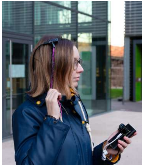
Figure 6.1: Interaction with FeatherHair in a public setting. The display in the hand depicts the recognized gesture.
