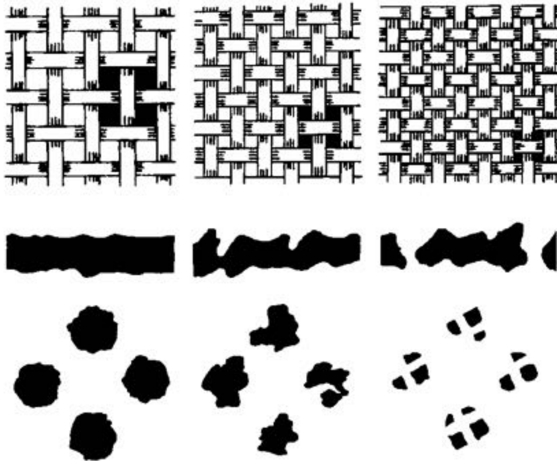
Figure 4.9: Varying mesh resolutions and the printing patterns, which result with increasing mesh resolution. Source: [Scheer 2007]
