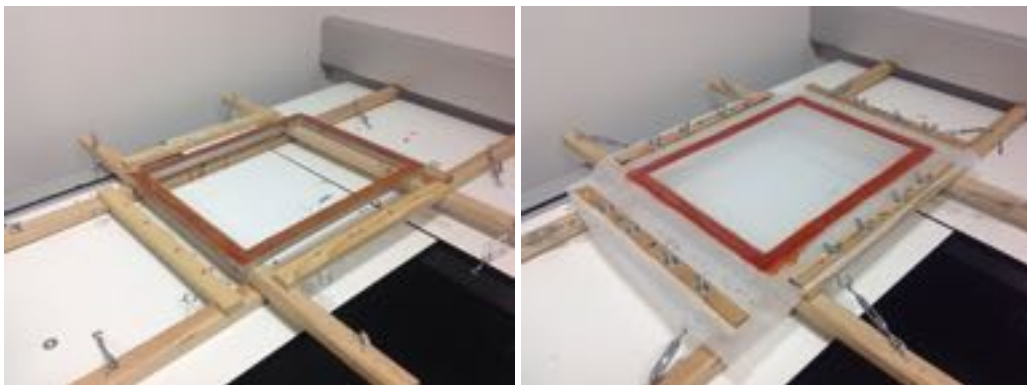
Figure 4.13: Stringing a net on a screen printing frame. Left: The frame is placed in the middle of the machine with the clamps parallel to the frame edges. Right: The net is stringed with the clamps and then glued on the frame.
