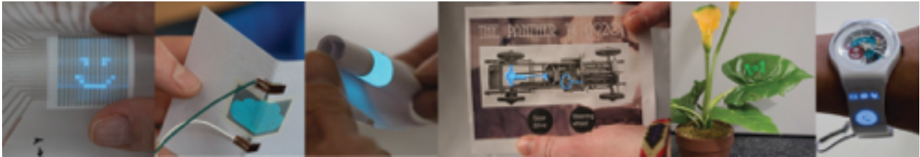
Figure 1. PrintScreen contributes a digital fabrication approach to enable non-experts to print custom flexible displays. They can be fully folded or rolled and enable manifold applications in ubiquitous, mobile and wearable computing.
