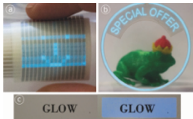
Figure 8. a) Passive Matrix Display. b) Translucent display on transparent PET film, in front of an object. c) Integration with laser-printed static visuals.
