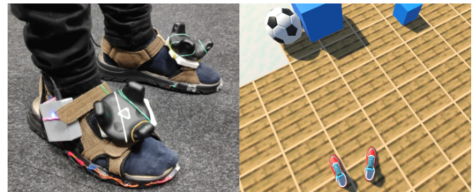
Figure 5. bARefoot prototypes augmented with HTC Vive sensors to track the positions of the user’s feet (left). First-person view of the VR application within which the user can experience walking on various virtual materials.
