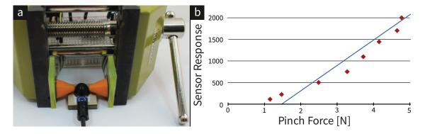
Fig. 6. Evaluation of pinch deformations: (a) apparatus; (b) sensor response for pinch forces with a fitted linear mapping function.
