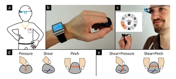
Fig. 1. (a) DeformWear enables expressive deformation-based input on various body locations: (b) One-handed input for smartwatches; (c) discreet input for head-mounted displays; (d) deformation primitives, and (e) their fluid combinations.
