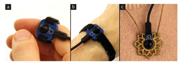
Fig. 2. Functional DeformWear prototypes: (a) ring, (b) bracelet, and (c) decorative pendant.
