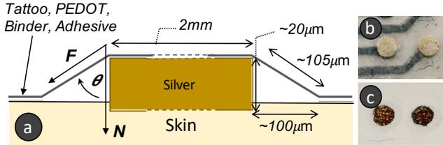
**Figure 3.** a) Micro-spring mechanism created by the tattoo substrate and the slightly thicker silver electrode; b) Micro-spring electrodes remain intact, while c) otherwise electrodes would deteriorate due to sparks.
