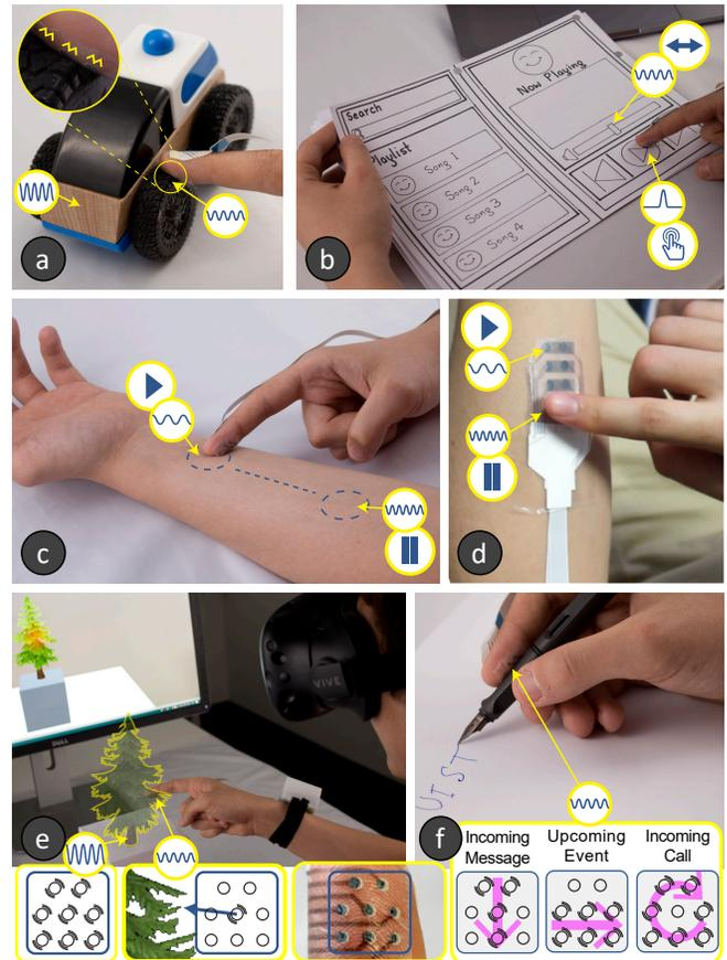
**Figure 5. Interactive example applications. a, b) Tactile augmented reality; c, d) Dynamic tactile landmarks for on-skin interactions; e) Tactile output in virtual reality; f) Private tactile notifications**
