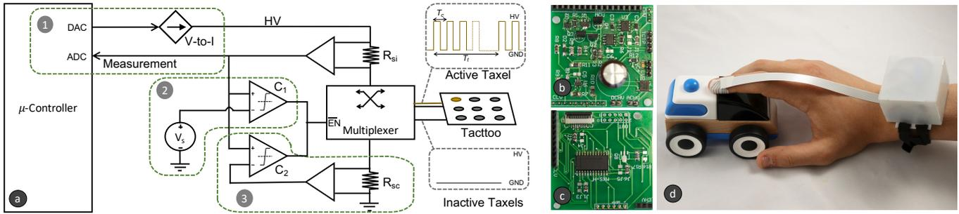
**Figure 4. Tacttoo control system; a) Three layer electrical safety architecture; b) Implementation of control and safety electronics; c) Modular multiplexing circuit which can be daisy-chained to increase the number of taxels; d) Complete mobile setup of Tacttoo with transferred tattoo, FPC connection and the control unit.**
