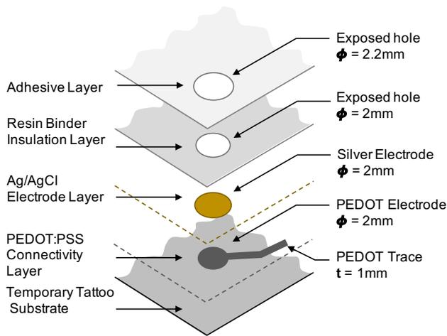
Figure 2. Layered fabrication of Tacttoo
