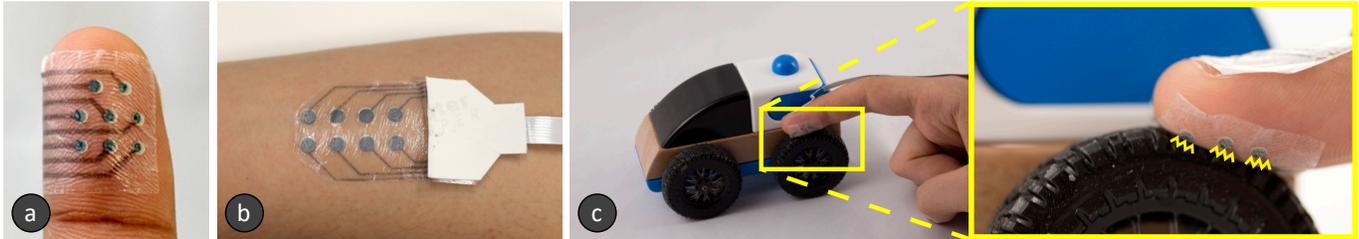
Figure 1. A Tacttoo rub-on tattoo enables feel-through and high-density tactile output. With less than  $35\mu\text{m}$  in thickness, it closely conforms to fine structures of the skin. Tacttoos can be custom-designed for various body locations and taxel densities, and fabricated using DIY tooling.
