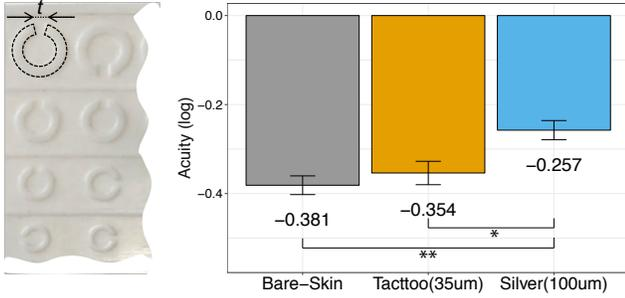
Figure 7. Ring chart used for acuity test and the results of the acuity test
