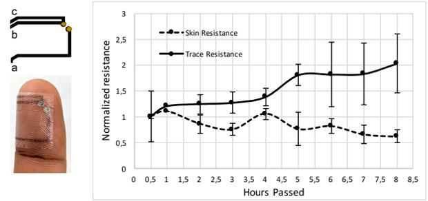
Figure 8. Durability test of Tacttoo. Overlay design (left) and normalized resistance over 8 hours (right)
