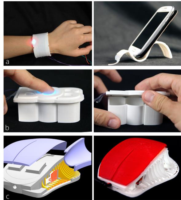
**Figure 15.** Application examples. a) An interactive shape-changeable bracelet. b) Interactive sealable treasure box with embedded TFEL display. c) Ergonomically customizable mouse: cutaway rendering and prototype after customization (cover removed to reveal deformation).
