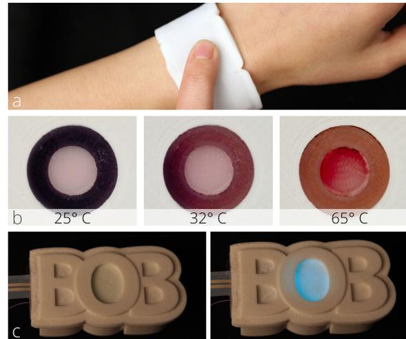
**Figure 3. Embedded input and output modalities: a) capacitive touch sensing, b) thermochromic display, and c) thin-film display.**
