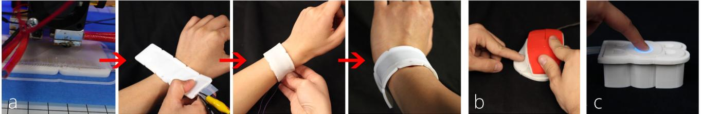
Figure 1. a) 3D-printed object with embedded state-changing elements. The end-user can physically customize the object on-demand after it is fabricated. This enables user-tailored wearables, b) ergonomically personalized devices, and c) new kinds of interactive objects.
