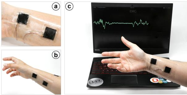
**Figure 5: Skin-exposed electrodes stencil painted with conductive paste onto gelatin (a, b) are used for EMG sensing (c).**
