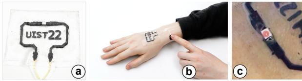
**Figure 3: Circuit (a) fabricated from a stack of three conductive alginate sheets using a plotter cutter. A surface-mount LED (a-c) can be driven at as low as 5V and controlled via a capacitive button (b).**
