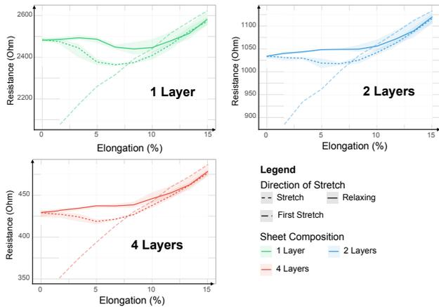
**Figure 10: Experimental measurements of resistance change under strain. We show hysteresis cycle graphs for samples of conductive alginate sheets with one, two and four layers.**
