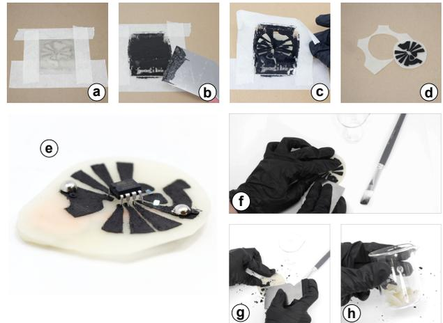
**Figure 7: Micro-controller shield (e) from beeswax with stencil painted carbon-based traces (a-d). At its end-of-life electronic components can be easily disassembled (f), traces scratched off (g), and the substrate molten and re-used (h).**
