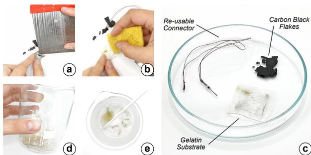
**Figure 6: The conductive water-soluble paste facilitates electrode disassembly (a, b) into re-usable connectors, carbon flakes, and gelatin scraps (c), which we can re-melt (d, e).**
