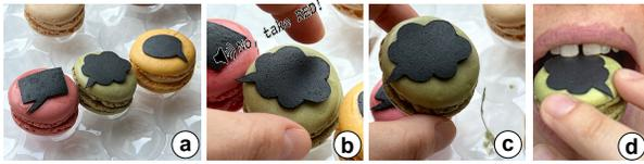
**Figure 4: Our pastry application case (a) uses conductive bioplastic sheets from gelatin and activated charcoal for 'speech bubble' capacitive proximity sensors (b-c). They have the potential to be edible (d).**
