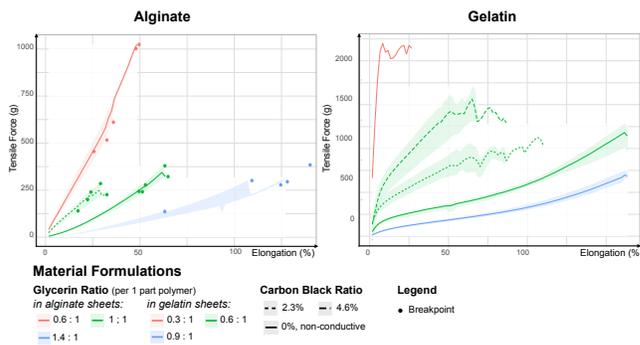
**Figure 9: Tensile strength measurements of conductive and non-conductive sheets from alginate (left) and gelatin (right). We compare different ratios of glycerin (stiff to flexible sheets) and carbon black (no, low and medium conductivity).**
