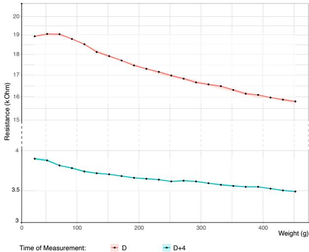
**Figure 11: Experimental measurements of resistance change that occurs when pressure is applied to the conductive foam. We report on repeated measurements of the same sensor, on the day of casting (D) and four days later (D+4).**
