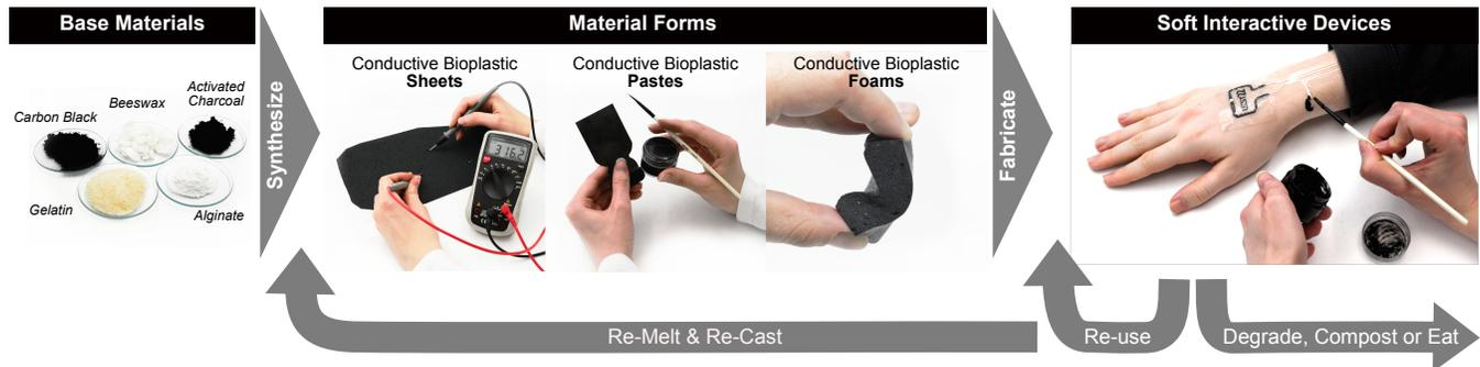
**Figure 1:** We synthesize conductive bioplastic sheets, pastes, and foams from sustainable base materials. Additive and subtractive fabrication methods allow to combine them with conventional electronics to create soft interactive devices. If no longer used, devices can be disassembled and parts re-used, materials re-molten and re-cast, bio-degraded, composted or eaten.
