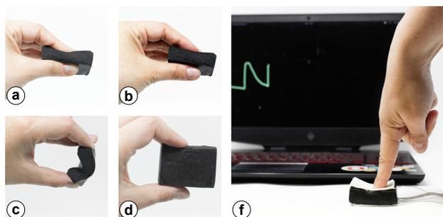
**Figure 8: A pressure sensor created from gelatin foam. The pressure sensor can be squeezed and freely deformed, reverting quickly to its original shape (a-d). Resistance changes caused by deformation can be read for pressure sensing (f).**
