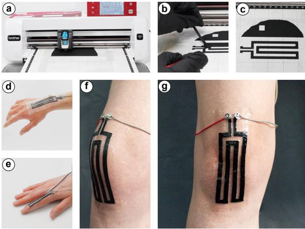
**Figure 2: Plotter cutting (a-c) allows to fabricate differently scaled bend sensors, e.g., to be placed on wrist (d), finger (e) and knee (f, g), out of carbon-infused alginate.**
