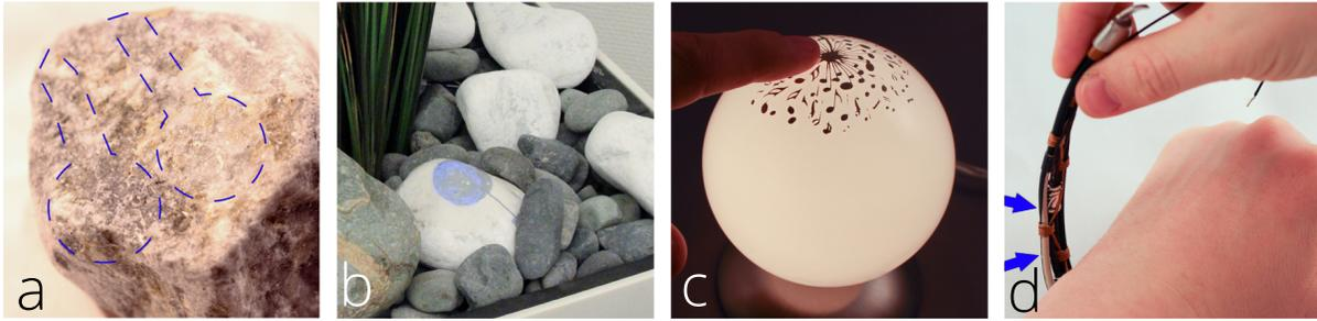
Fig. 10. Augmented everyday objects for novel interactions. A rock is augmented with two translucent electrodes (marked with dashed lines), leveraging two areas of distinct roughness for eyes-free interaction (a). Prototyping interaction on unconventional everyday objects: a garden stone (b), a glass lampshade (c), and a leather bracelet (d, electrodes at arrows).
