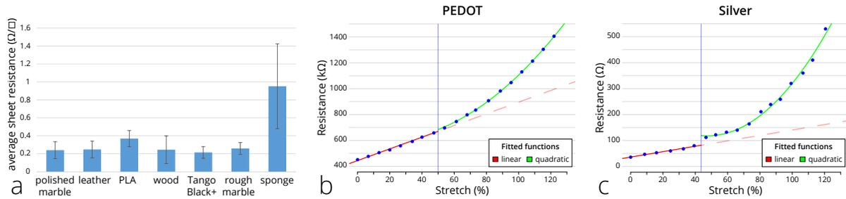
Fig. 4. Evaluation results: a) Sheet resistance on different materials using the high-fidelity approach. b) and c) Change in resistance by stretching for PEDOT and silver ink respectively. Trends are indicated by a fitted linear model (red) for data points below the blue line and quadratic fit (green) for points above. The dashed red line illustrates the continuation of the linear model.
