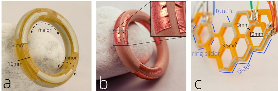
Fig. 9. Prototyping geometry-guided touch gestures. A wooden ring (a) is augmented with 9 conformal electrodes to support circular gestures following its major and minor radii. In contrast, adhesive copper tape causes wrinkles due to the non-developable geometry and edges due to its thickness (b). A honeycomb pendant (c) illustrates three geometry-guided touch interactions.
