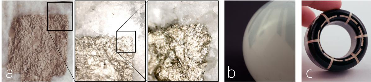
Fig. 6. Printed electronics transferred with the proposed approach conform closely to highly curved non-developable geometries. a) Silver conductor conforming to a rough stone surface (image of  $1\text{cm}^2$  patch and magnification of selected area). b) Translucent PEDOT conductor conforms to white glass sphere without distortion. c) Silver traces wrapping into hollow cylinder geometry.
