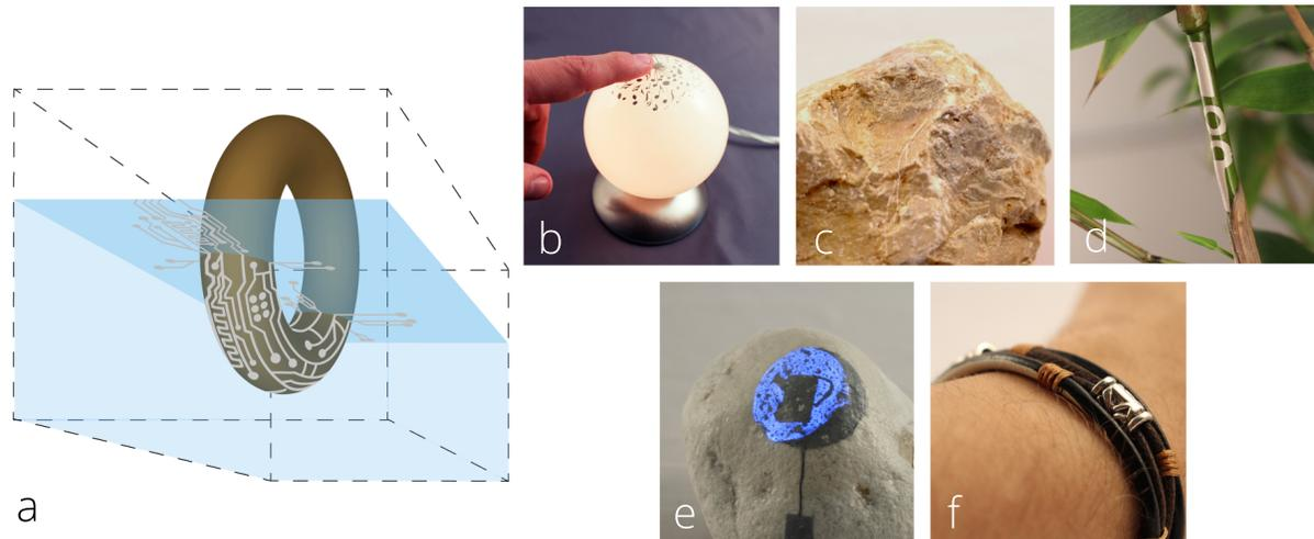
Fig. 1. ObjectSkin is a fabrication technology for adding interactive surfaces to everyday objects (a). It is used to realize custom sensors and displays that seamlessly conform to highly curved geometries (b) and the detailed surface structure (c) of a wide variety of everyday objects, including live plants (d), garden stones (e), and aesthetic wearables (f).
