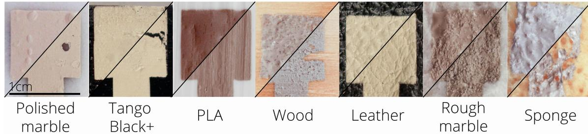
Fig. 3. Materials. Top left: sample covered with transparent PVA transfer film, bottom right: after washing the PVA transfer film off.
