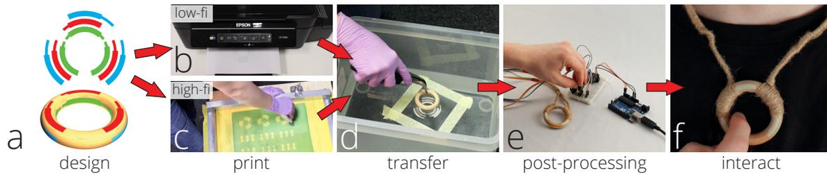
Fig. 2. ObjectSkin fabrication process. The digital design (a, color indicates mapping) is printed using the low-fidelity inkjet-based (b) or high-fidelity screen printing (c) approach onto a PVA transfer film. The object is dipped through the printed ink and dissolved transfer film, allowing the ink to conform to the object (d). After post-processing and connecting to a microcontroller (e), the prototype is ready for interaction (f).
