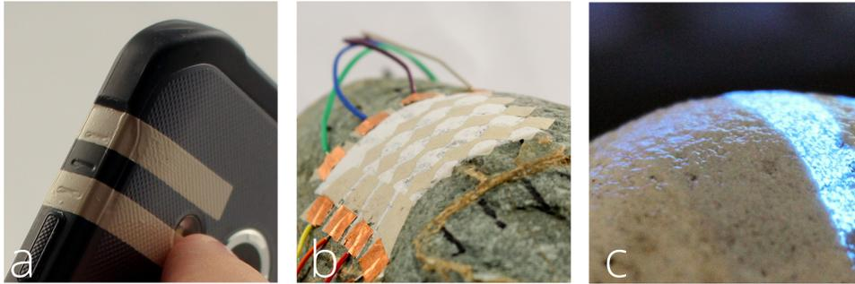
Fig. 8. Conformal sensors & displays: touch extension on smart phone (a), multi-touch matrix on rock (b), and electroluminescent display on stone (c).
