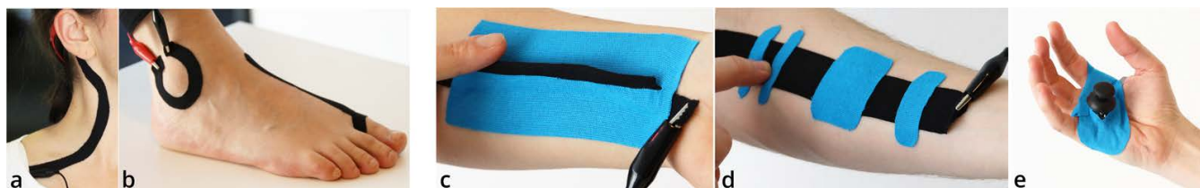
Figure 3: Kinesiomy tape allows for a large variety of on-skin placements, including areas with non-uniform curvature, such as around the neck (a) or bones (b). The combination of non-resistive (blue) and pretreated (piezo-resistive, black) kinesiomy tape allows using ridges and folds (c), partitions (d), and electronic components (e).
