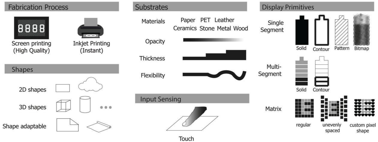
Figure 2. Five-dimensional design space for digital fabrication of customized displays.
