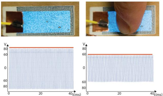
Figure 9. Touch sensing. The amplitude of the AC signal drops when the segment is touched.
