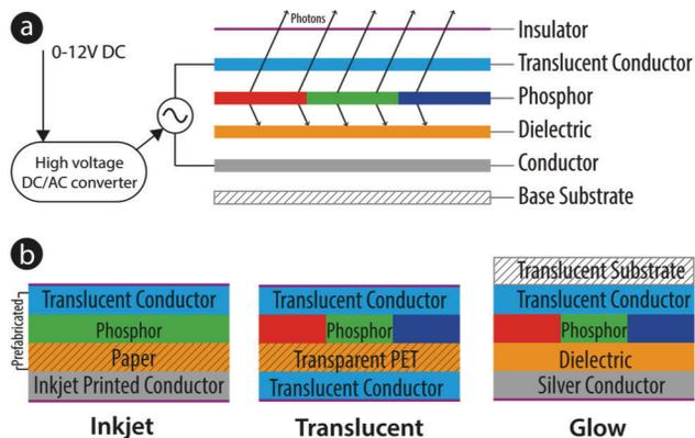
**Figure 3. a) Composition of the printed layers of an electroluminescent display: Silver Conductor (C2131014D3, 100mΩ/sq), a barium titanate based dielectric (D2070209P6), phosphor (e.g. C2101125P4) and a PEDOT based translucent conductor (D2070209P6, 500-700 Ω/sq). b) Variations of the standard structure to create translucent displays, display glowing through materials or inkjet-printable displays.**
