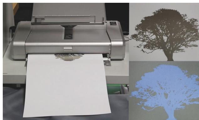
**Figure 5. Instant inkjet printing. A printed electrode (left, upper right) is illuminated (lower right).**
