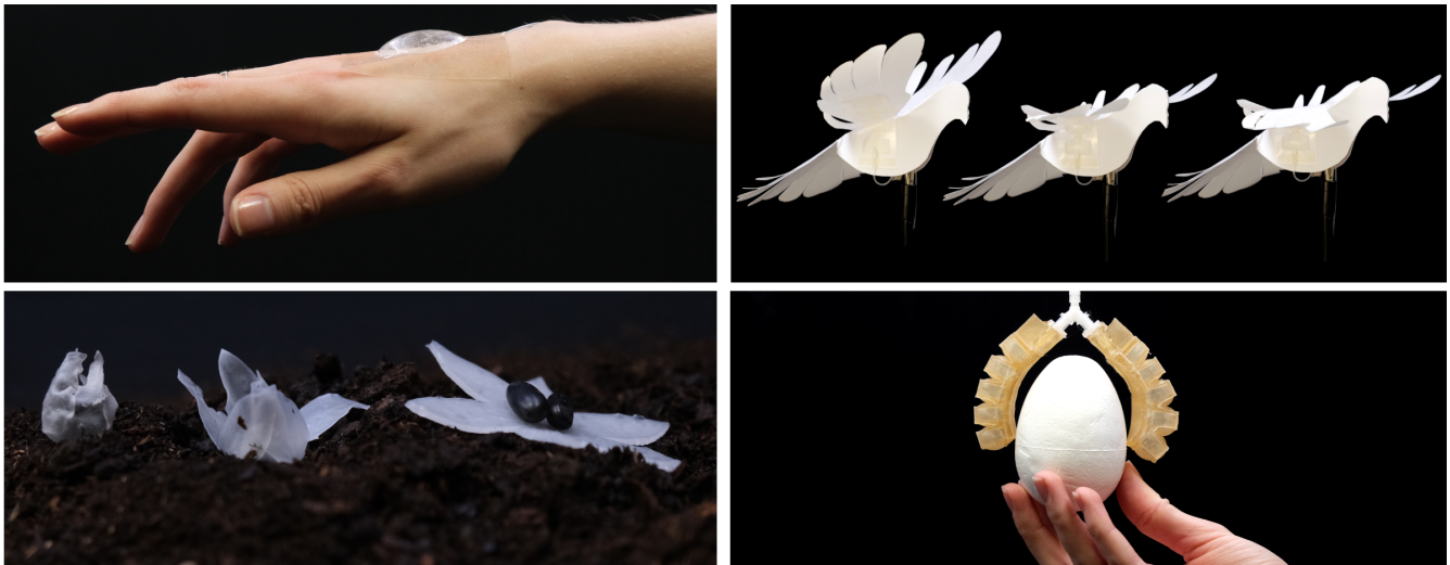
Figure 1: We showcase four out of our five case studies: from top left to bottom right, an epidermal notification interface, a biodegradable seed dispenser, a mechanical bending actuator on a paper bird, and a replication of the soft pneumatic gripper [63]. ©Madalina Nicolae
