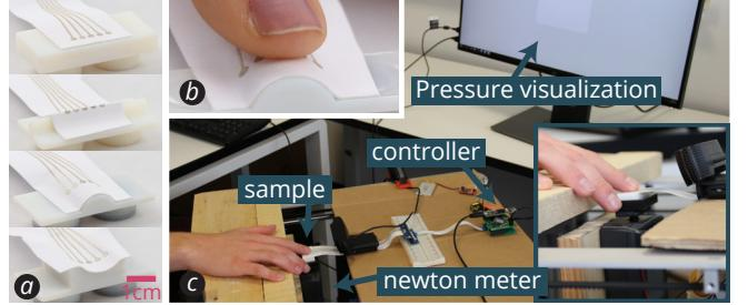
**Figure 11.** Study overview: (a) planar, convex and concave geometries used; (b) finger on convex curved geometry, and (c) study setup.
