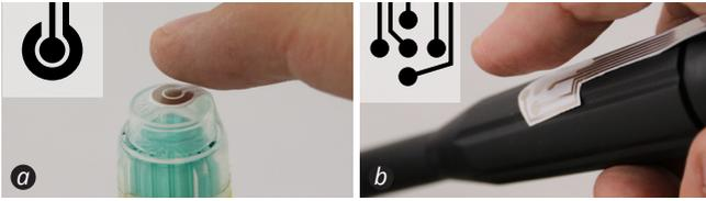
Figure 7. Two printed button Tactlets placed on curved geometries: (a) enable/disable button and (b) pattern button.
