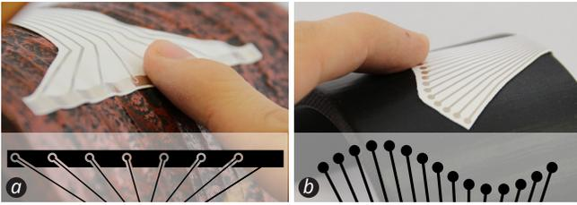
Figure 9. Two printed slider Tactlets with (a) lower and (b) higher taxel resolution placed on curved geometries.
