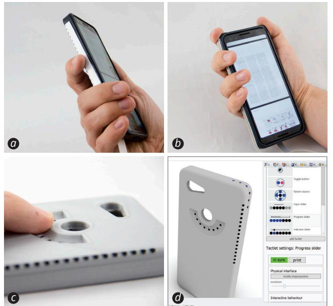
**Figure 13. Application case 1:** Through several iterations different slider Tactlets are quickly prototyped on a smart phone case. (a) A long slider on a curved edge on the back of the case, (b) a short slider wrapped around the top left curvature, and (c) a curved concave slider on the back of a 3D-printed prototype. (d) All Tactlets are digitally designed in the design tool.
