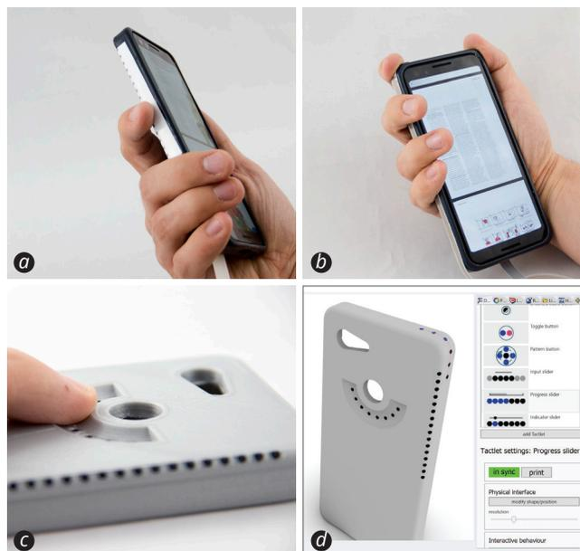
**Figure 13. Application case 1: Through several iterations different slider Tactlets are quickly prototyped on a smart phone case. (a) A long slider on a curved edge on the back of the case, (b) a short slider wrapped around the top left curvature, and (c) a curved concave slider on the back of a 3D-printed prototype. (d) All Tactlets are digitally designed in the design tool.**
