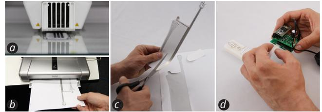
**Figure 4. Rapid fabrication example:** The designer prints the physical prototype on a 3D printer (a). Alternatively, she prints the interface on a conductive inkjet printer (b), cuts it out (c), and attaches it. Finally, the prototype is connected to the Tactlets controller (d). The entire fabrication (b-d) of the presenter prototype takes less than 5 minutes.
