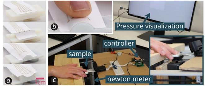
**Figure 11. Study overview:** (a) planar, convex and concave geometries used; (b) finger on convex curved geometry, and (c) study setup.
