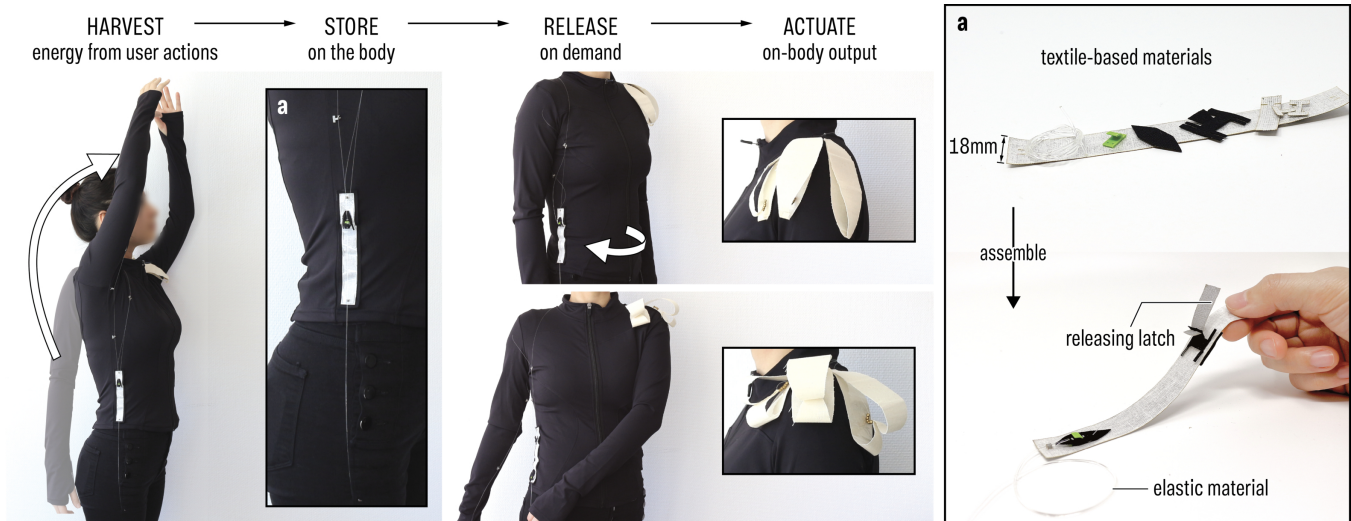
Figure 1: Texergy enables more interactive and programmable passive on-body actuation by "powering" the actuation with mechanical energy that is harvested from innate user actions, stored on the body, and later released on demand. For example, this shape-changing costume is powered implicitly by dance moves to actuate a dramatic visual effect that amplifies the performance. (a) Texergy mechanisms are made with textile-based materials and a digital fabrication process, enabling seamless integration into the clothing and customization.
