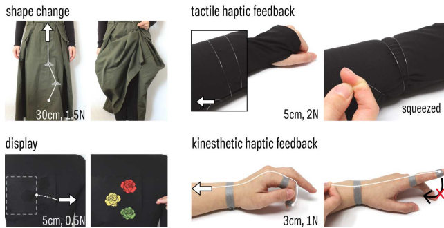
Figure 6: Example string-based output end-effectors that enable creating a shape change, a display, and tactile and kinesthetic haptic feedback.
