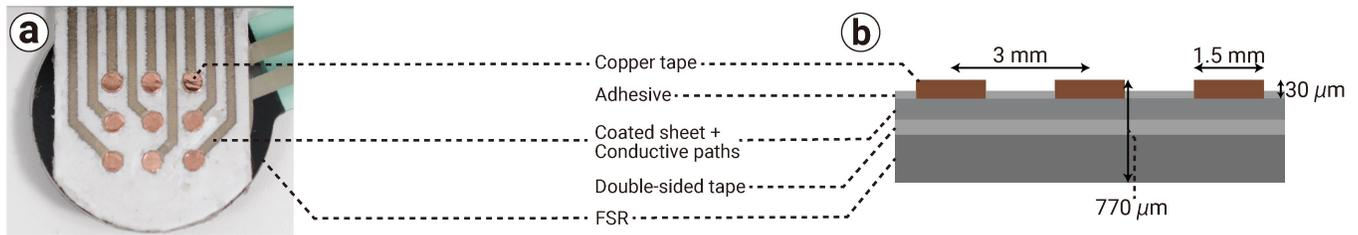
**Figure 3: Our finger-worn interface comprises (a)  $3 \times 3$  electrodes and an FSR. (b) They are stacked with double-sided adhesive tape.**
