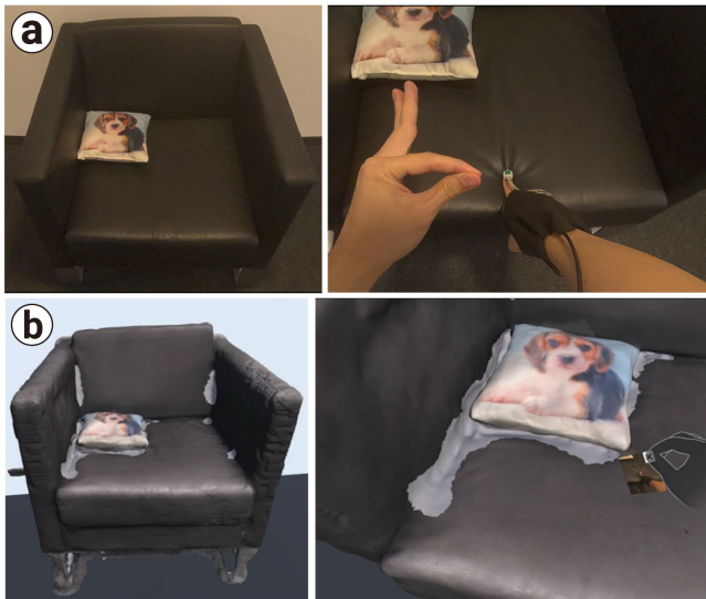
Figure 8: HapticPipette enables remote users to share their haptic experiences. The user (a) captures the compliance of their sofa and (b) applies it to a 3D reconstructed mesh in a collaborative VR environment, which other users can interact with.
