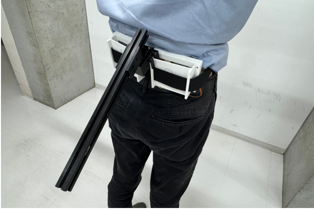
Figure 13: Prototype integrating a 1-DoF robotic tail with the Imaginary Joint device.
