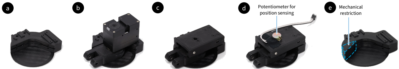
Figure 9: ExoKit features interchangeable joints based on a versatile joint base (a). This base can be fitted with (b) a motor for actuated joints, (c) a passive module to replace the motor, or (d) a passive module with an integrated position encoder for sensing-only joints. (e) Designers can insert mechanical restrictions to the base joint to further limit the offered range of motion by 15, 30 or 45° on each side.
