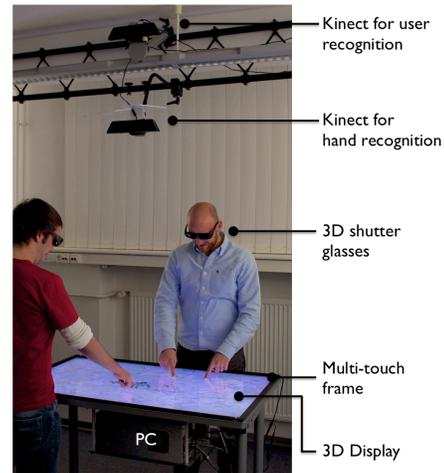
**Figure 2. Prototypical implementation of Permulin**
