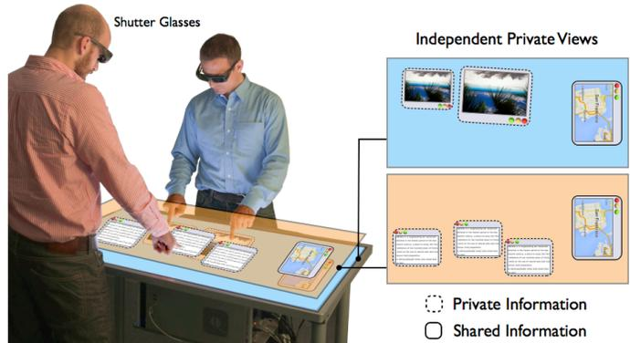
**Figure 1. The multi-view tabletop provides distinct private views or a group view that is overlaid with private contents. Our techniques provide support for easy and seamless transitions along the entire spectrum between tightly coupled and loosely coupled collaboration.**
