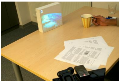
Figure 8. A photostream from Flickr is projected onto a box and can be navigated by rotating the coffee mug.
