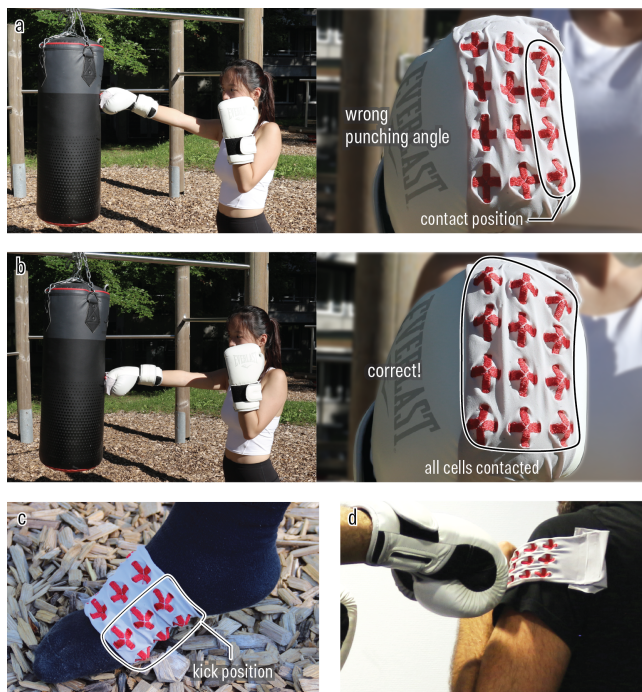
Figure 22: We design a user-triggered shape display for visualizing contact in boxing training. (a) Contacted structures pop out to tell the contact position such that the users can (b) adjust their postures and get immediate feedback. The patch can also flexibly wrap around different body parts for (c) kicking and (d) dodging exercises.
