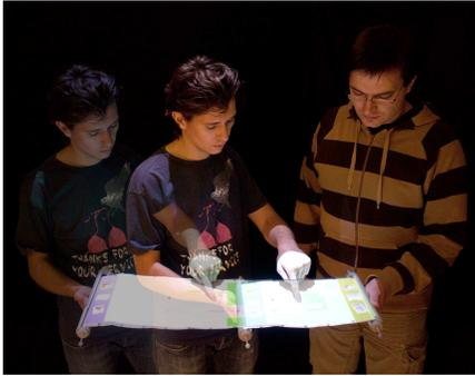
**Figure 1.** A mobile device with a rollout display can act as a large interactive surface on-the-go. The surface can be dynamically resized to adapt to the demands of different collaborative settings.
