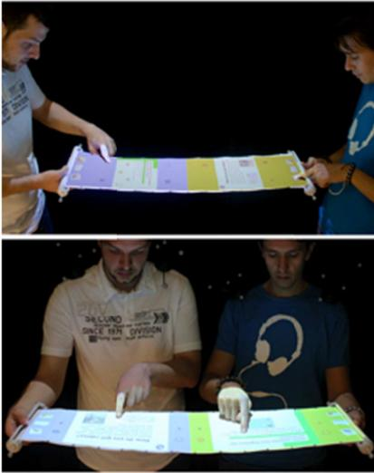
**Figure 9.** Splitting-up into sub-activities by moving to the vis-à-vis portrait or side-by-side formation. The display is automatically split into separate personal zones.
