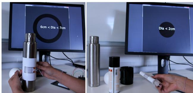
Figure 8. Curvature measurement using a single sensor
